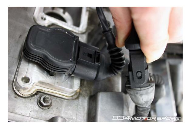
The supplied FSI coil connector adapters are long enough to allow you to tuck the new coil plug junction out of the way, or under/behind the runners of the intake manifold. Installing them behind the intake manifold runners requires unclipping some of the fuel injector connectors for easier access. Make sure you plug them back in.
