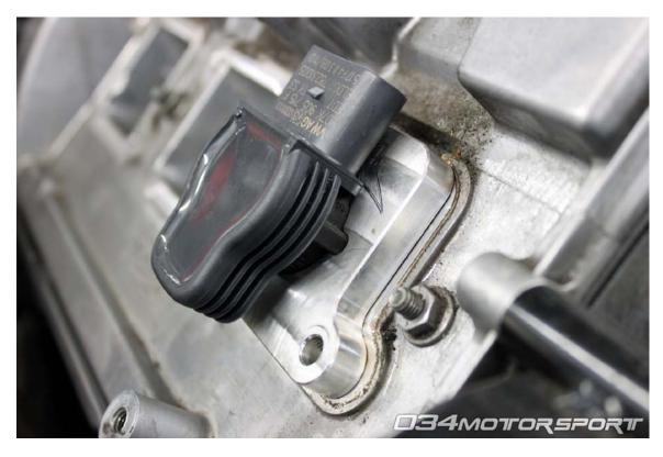
Once all the coils have been installed, it is time to install the 034Motorsport FSI coil connector adapters. The 4-wire side plugs into the coil; make sure it clicks to indicate it's fully seated and locked. Next, plug the 3 wire side to your original coil connectors.
