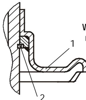
**When fitting the spring plate ( 1) care must be taken to ensure that the circlip ring ( 2) is seated correctly!**
