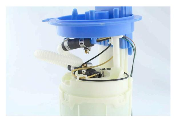
9 – reinstall the assembly into the fuel tank and attach a length of hose to the outlet of the pump assembly allowing it to drain into a fuel safe container and prime the fuel pump assembly
