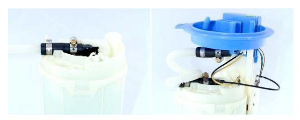
8 – reinstall the top and connect the wires to the DW65v
